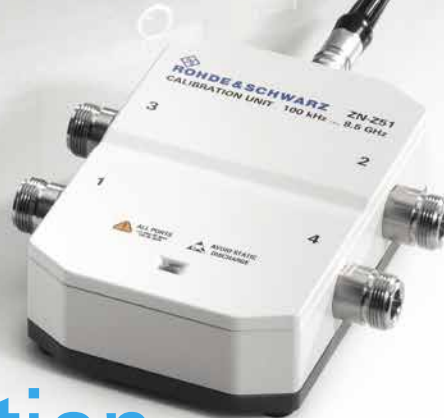
Fig. 1: The R&S®ZNB vector network analyzer with the R&S®ZN-Z51 automatic calibration unit (N (f) connector).
