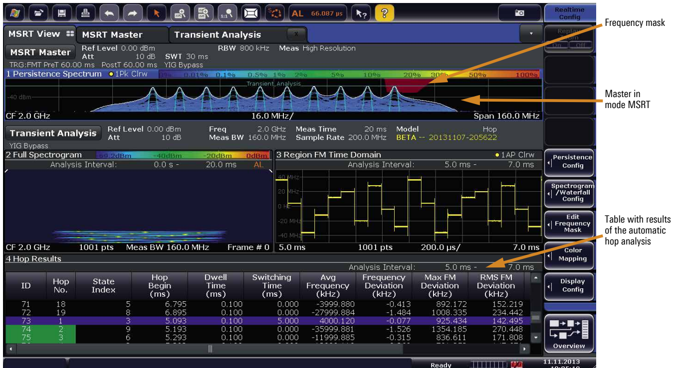
Fig. 6: The frequency mask trigger is defined in the realtime spectrum analyzer (top). Automatic analysis of the hop sequence (bottom) takes place in the R&S®FSW-K60 transient analysis option.
