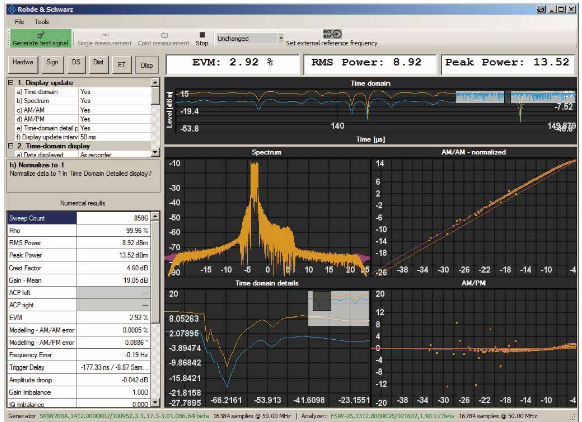
Fig. 6: Measurement of the AM/AM and AM/PM conversion as well as of EVM, peak and RMS power of an LTE UL signal using the R&S®FSW amplifier characterization software application.
