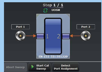
Fig. 4: The calibration menu on the R&S®ZNB vector network analyzer with the selected calibration unit.
