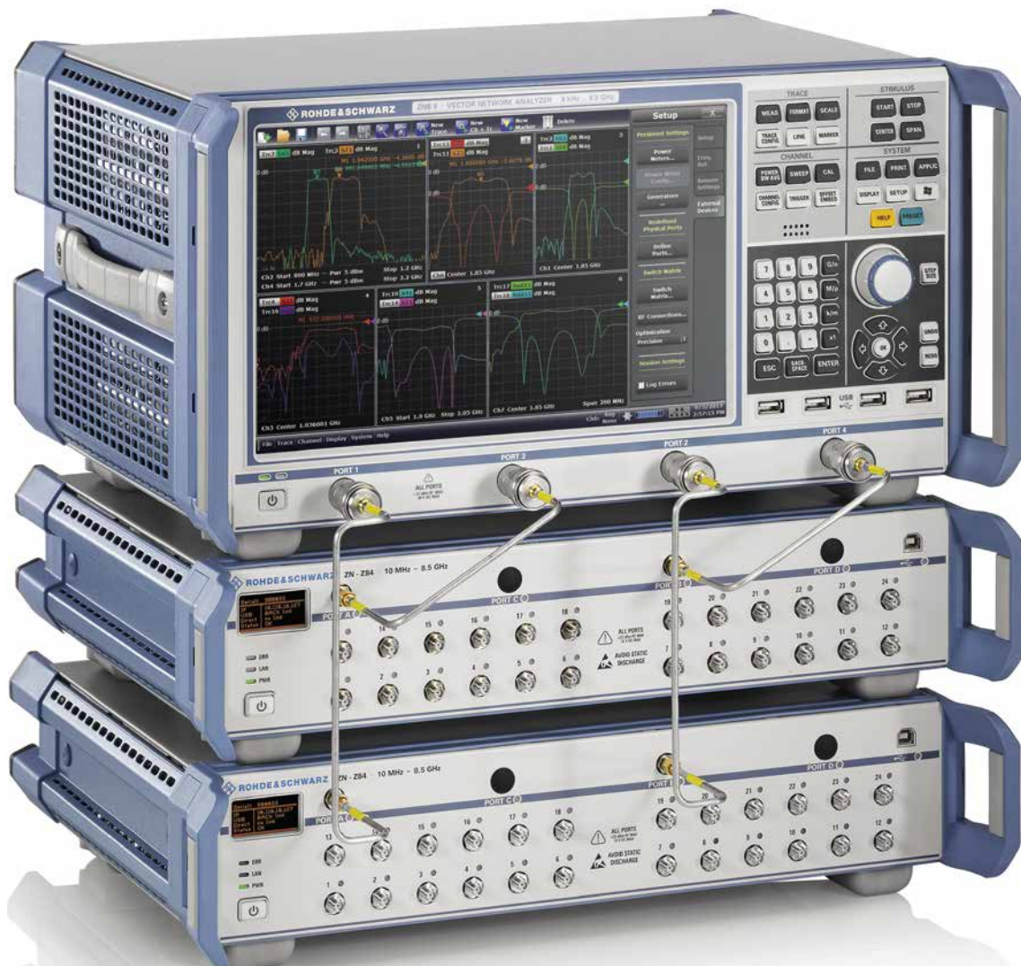
Fig. 1: The R&S®ZNB vector network analyzer with two R&S®ZN-Z84 switch matrices provides up to 48 ports.
