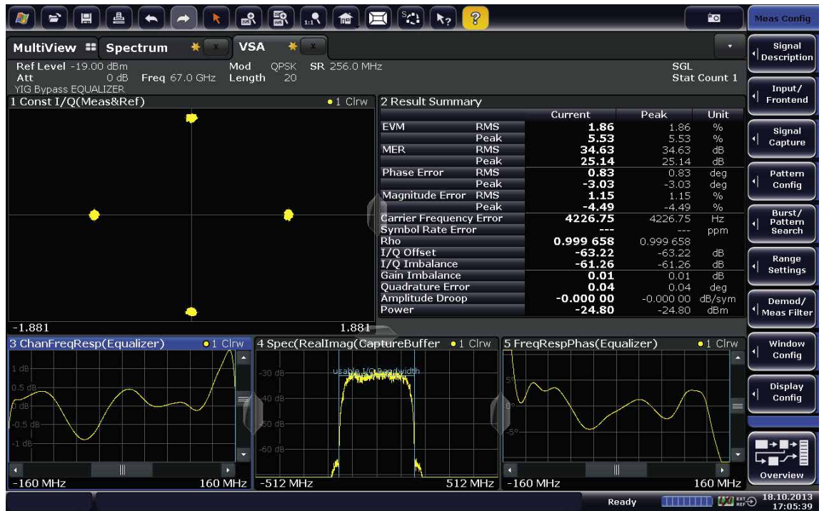
Fig. 2: Example of an EVM measurement on a QPSK signal with a 256 MHz symbol rate at 67 GHz.
