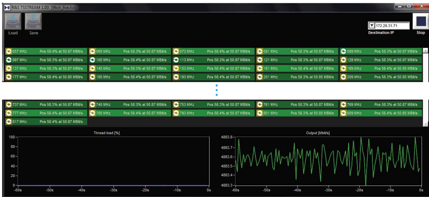
Fig. 1: The R&S®TSSstream streaming view displays the status of all generated IP streams, computer workload and total generated data rates at a glance.
