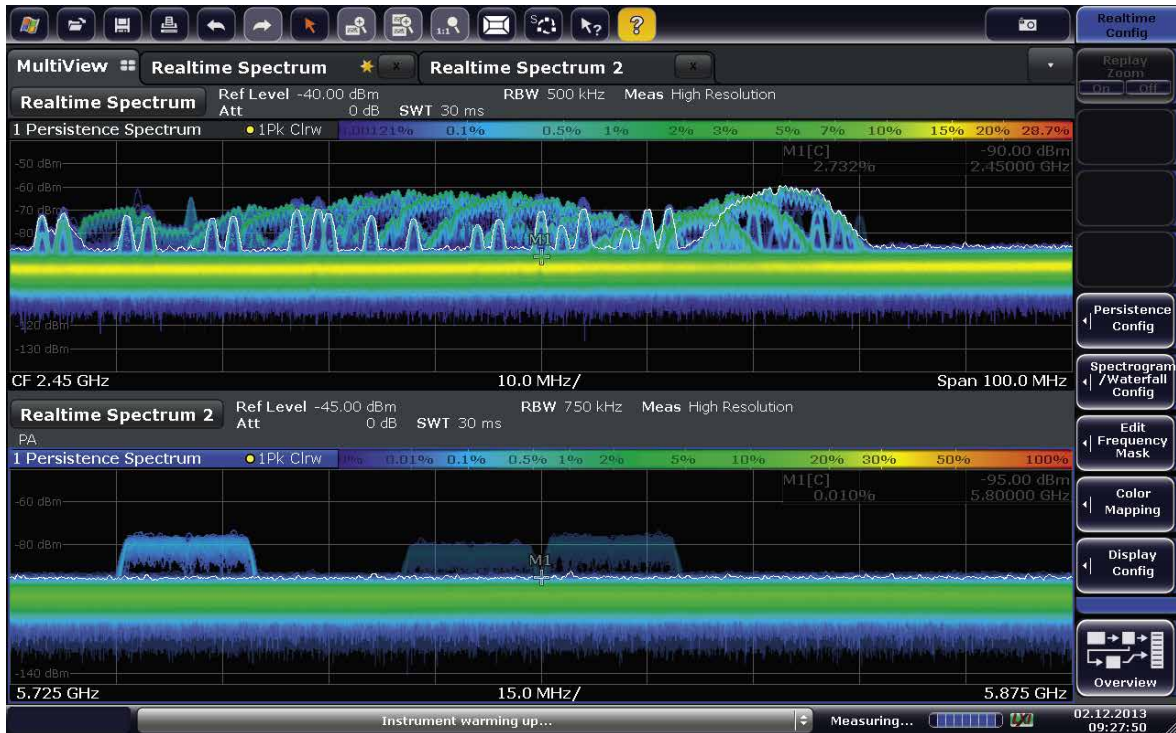
Fig. 7: Two ISM bands in one display. Top: The 5.6 GHz ISM band, where only devices that are compliant with WLAN standard 802.11n are active. Below: The 2.4 GHz ISM band is at the bottom of the display, in which both Bluetooth® and WLAN signals can be seen.
